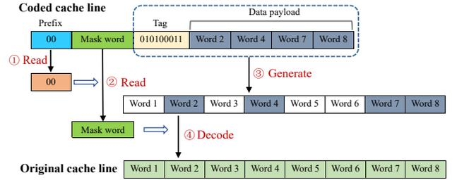
Fig. 7. Read procedure of SimiEncode
