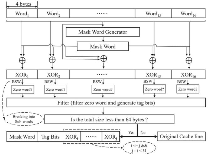
Fig. 11. Implementation of a 4-byte granularity encoder unit to encode a 64-byte cache line.
