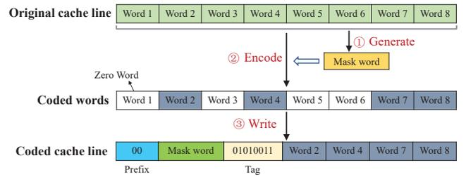
Fig. 6. Write procedure of SimiEncode.
