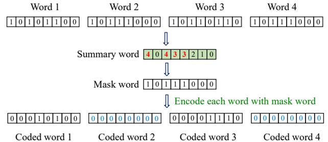
Fig. 3. An encoding example of SimiEncode.
