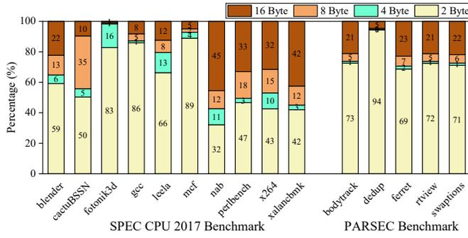
Fig. 5. The proportion of zero words generated by different encoding granularities.
