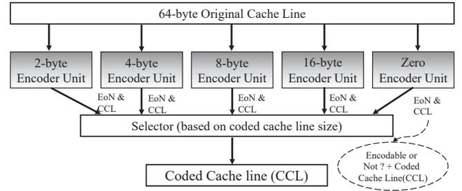
Fig. 10. The encoding logic consists of 5 separate encoder units.
