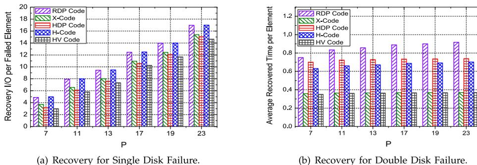
(a) Recovery for Single Disk Failure.
