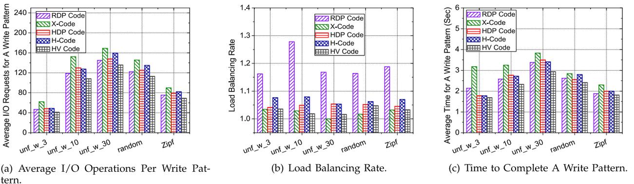
Fig. 8. Partial stripe write efficiency in reconstruct-writemode ( $p = 13$ ).
