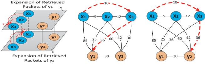
(a) Expansion: the cost is 37. Each link will transmit one packet. (b) Aggregation of  $y_1$ : the cost is 92. Each link will transmit two packets. (c) Aggregation of  $y_2$ : the cost is 92. Each link will transmit two packets.
