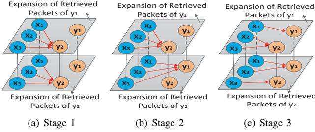
Fig. 4. The selection of expansion nodes ( $r = 2$  and  $d = 3$ ). (a)  $y_2$  is the common expansion node of all the retrieved packets. (b) The retrieved packets of a newcomer will choose the same expansion node. (c) Different retrieved packets can have different expansion nodes.
