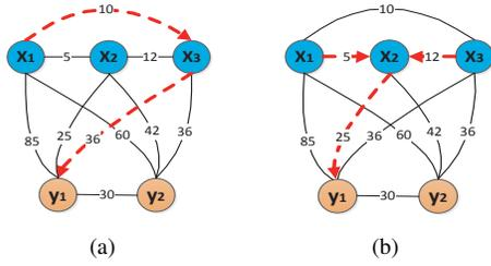
Fig. 3. Two Steiner Trees constructed over  $\{y_1, x_1, x_3\}$ , where  $\{x_1, x_3\}$  are expansion nodes and  $y_1$  is a newcomer.
