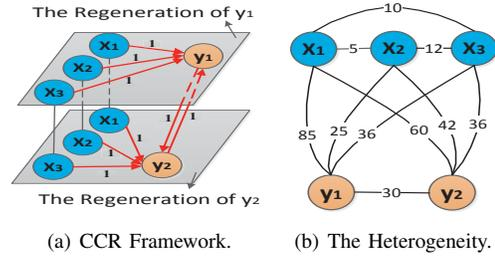
Fig. 1. The cost of CCR framework in a heterogeneous environment. The arrow shows the number of transmitted packets. The total cost is 344.
