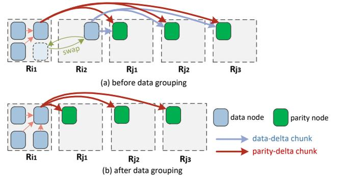
Fig. 4. Data grouping: we can swap the updated data chunk in  $R_{i2}$  with one of the chunks in  $R_{i1}$ , such that the four updated data chunks are now stored in  $R_{i1}$ .
