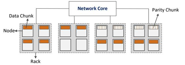
Fig. 1. A DC that comprises four racks with four nodes each. Suppose that the DC employs RS(14,10) for erasure coding. It may distribute the data and parity chunks of a stripe across 14 different nodes that reside in the four racks.
