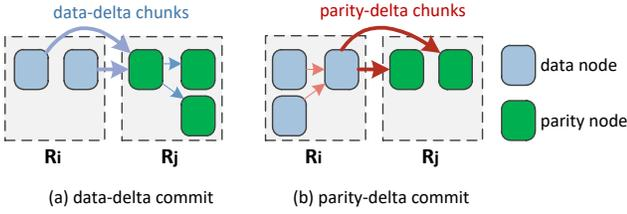
Fig. 3. Selective parity updates: (a) data-delta commit and (b) parity-delta commit. In (a), CAU sends  $i' = 2$  data-delta chunks from  $R_i$  to  $R_j$ ; in (b), CAU sends  $j' = 2$  parity-delta chunks from  $R_i$  to  $R_j$ .
