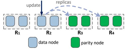
Fig. 5. Interim replication: we store two replicas of a newly updated data chunk (resided in  $R_2$ ) in two racks (i.e.,  $R_3$  and  $R_4$ ), in order to guarantee the reliability of the newly updated data chunk against any double rack failures.
